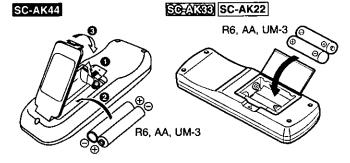
Insert the batteries observing the correct polarities  $(\oplus, \Theta)$ .
